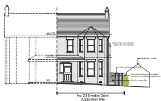
PROPOSED SOUTH (FRONT) ELEVATION 1:100
