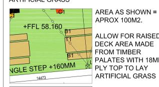
APROX 100M2. ALLOW FOR RAISED DECK AREA MADE FROM TIMBER PALATES WITH 18MM PLY TOP TO LAY ARTIFICIAL GRASS
